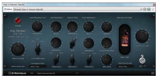
Fig. 3. The included Pultronic EQ emulates a four-band Pultec, and adds character to your sound in a way that more conventional, surgical parametric EQs can't.
