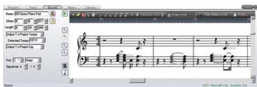
Fig. 2. You can show and edit MIDI notes using a standard piano-roll screen, or choose per-track notation.
